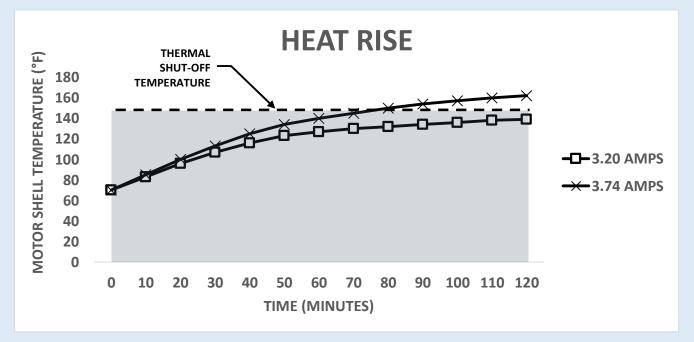
The Shaded area in the charts above indicate performance points where pumps are capable of running without periodic cool down based on current draw. Pumps in the unshaded areas require periodic shut down for motor cooling. Some applications require maximum flows at high pressures for relatively short periods, so an explanation of thermal protection follows:
